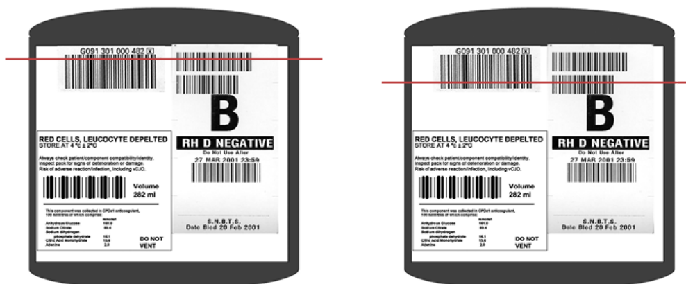
Figure 23.2: Two concatenation processes. On the left the donation identification number (DIN) with nationally defined structure, and on the right the DIN with the ABO/Rh blood group barcode.
