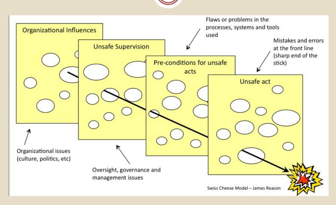
Many layers of defense usually lie between hazards and accidents but there are flaws in each layer which if aligned can allow the accident to occur.
