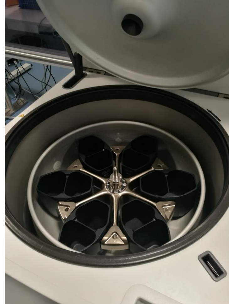
Blood centrifuge spins at between 3150 and 3840 times a minute!
